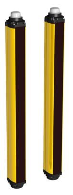
Banner SGS Safety Grid System is a two-piece (emitter and receiver), redundant, microprocessor-controlled, opposed-mode optoelectronic "light grid". Standard models are available in 2 beam (500 mm beam spacing), 3 beam (400 mm beam spacing), or 4 beam (300 mm and 400 mm beam spacing) systems.
